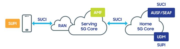
Through encryption and home authentication, the 5G network increases protection of the device and preserves the integrity of the network by only allowing access to authentic users. The 5G network now both enhances the authentication process and eliminates sending the user device's unprotected identity, preventing the theft of the ID by cyber criminals.
